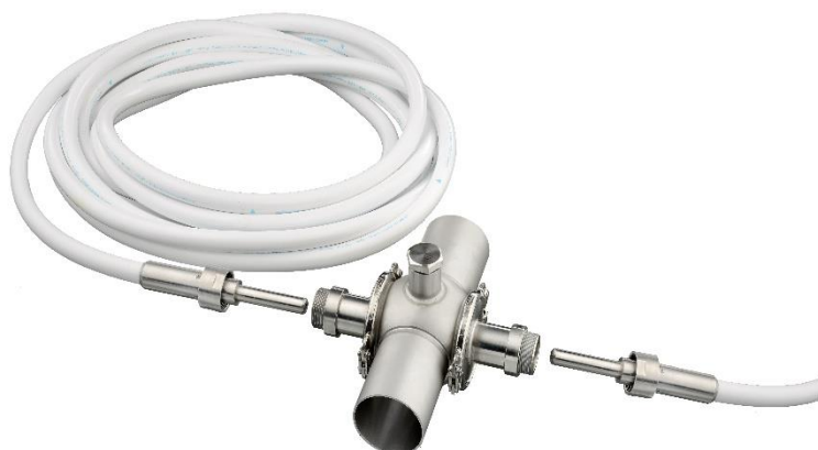
Figur 23: Transmissionsmålecelle m 1,0 mm åbning.
