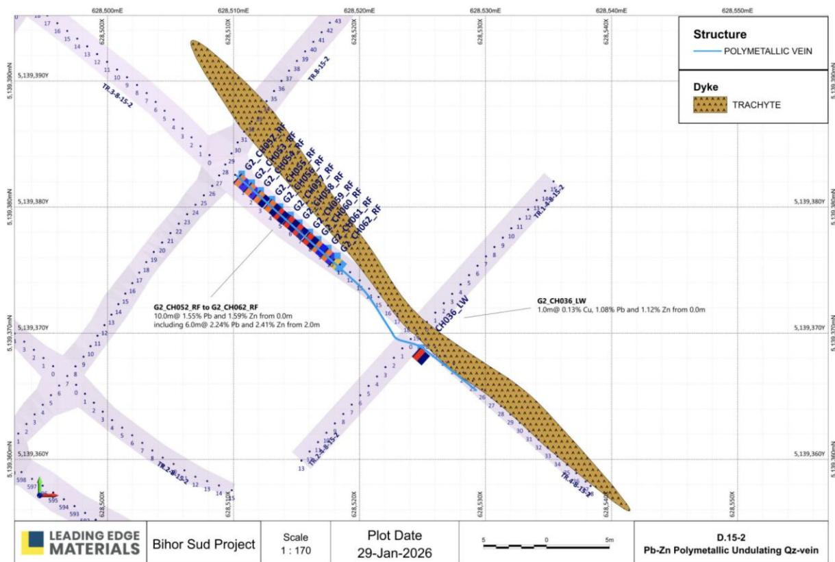
**Tr.35-21-2 and Tr.33-21-2: the mineralisation observed in this area appears to be controlled by several faults with variable dip, extending toward the SW and NE. Mineralisation has been confirmed along faults with a NW-SE strike length of approximately 90 metres and possible widths of up to two metres. The system remains open in all directions.**
