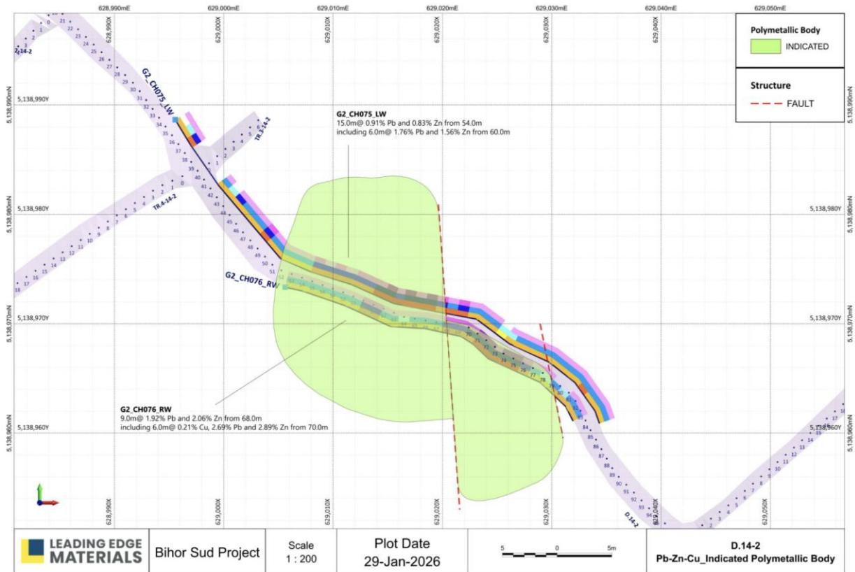
**Tr.5-20-15-2:** Extensive Pb-Zn-Cu mineralisation associated with silica alteration along a NNW-SSE strike. Presence of an earlier dyke that intersects the system has possibly caused structural displacement of the mineralisation. The system remains open along strike and down-dip, extending towards the SW.
