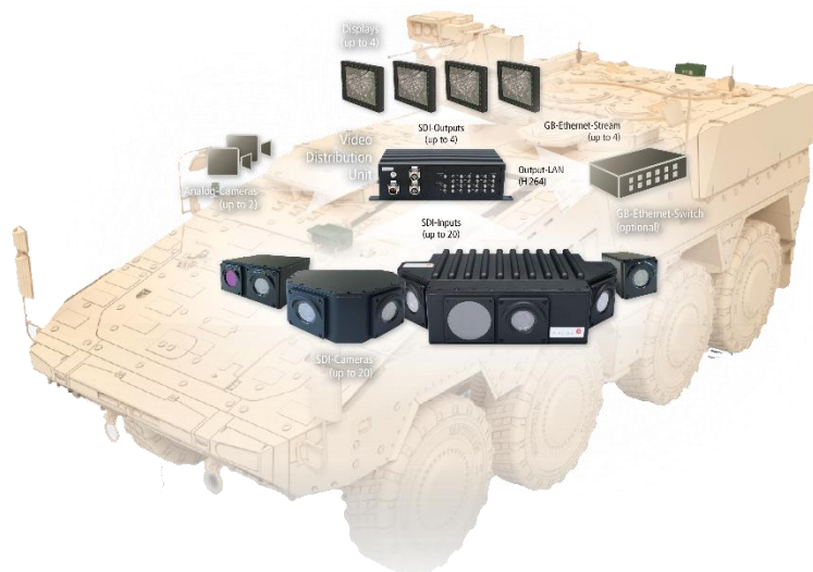
KAPPA's scheme of System Composition for Tanks
