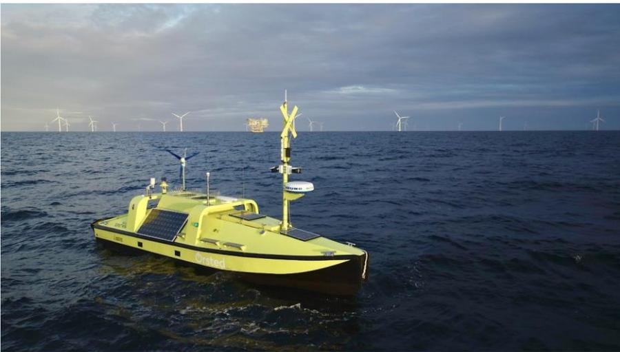
**Ørsted, the world's leading developer of offshore wind farms, has designed and developed the first uncrewed surface vessel (USV) in the industry for offshore met-ocean measurement campaigns. The measurement data will help lower uncertainties in the expected annual energy production for new offshore wind farms. Ørsted, who has patented the USV concept, sees enormous potential in the technology and has initiated a serial production based on their successful prototype USV.**
